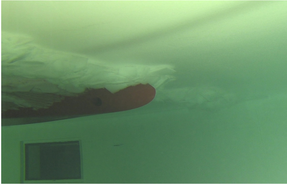
Figure 28: Reference ship penetrating through a small ridge
