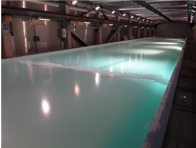
Figure 15: Triangular ridge in level ice field
