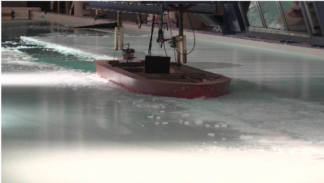
Figure 30: Attempt to break out from channel with Reference ship
