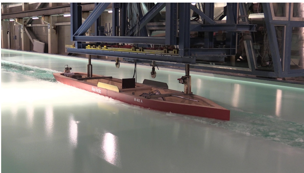
Figure 31: Attempt to break out from channel with EEDI bow
