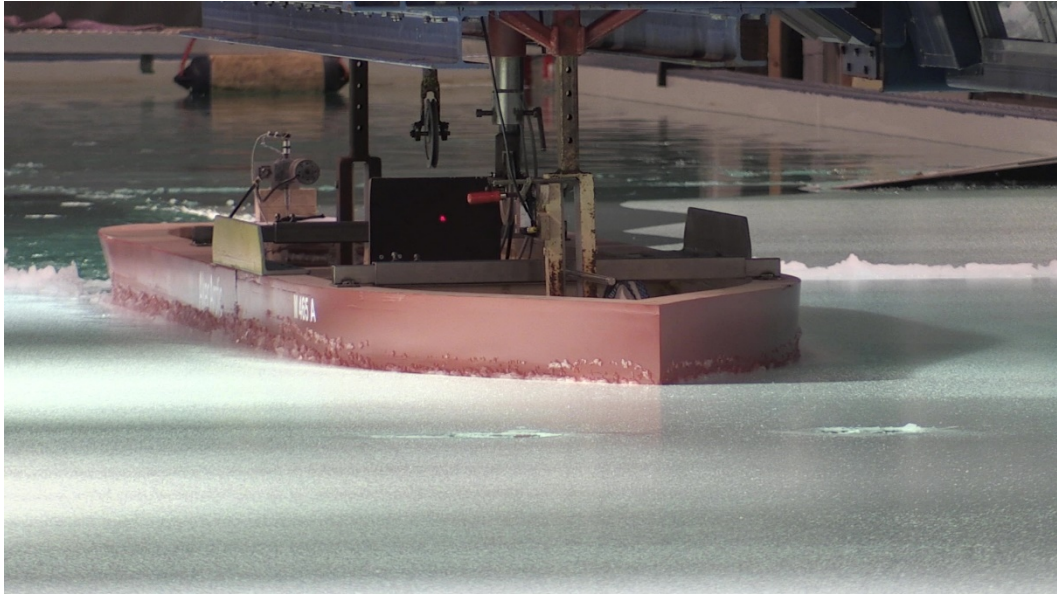
Figure 20: EEDI bow breaking the ice, in this case, by crushing and cutting
