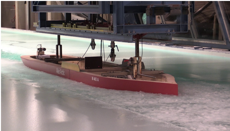
Figure 23: FSICR IA brush ice channel, EEDI bow
