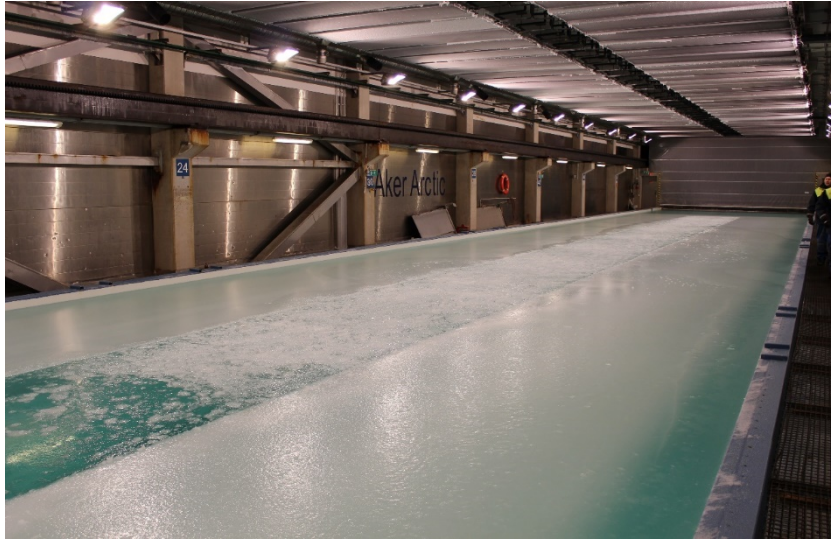
Figure 13: Brash ice channel, ice class IA
