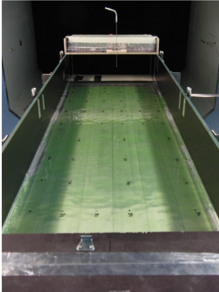
Figure 3-8 Fluid layer on the FPET duct floor. Markings indicating the measurement points of the fluid thickness and the surface temperature are visible.
