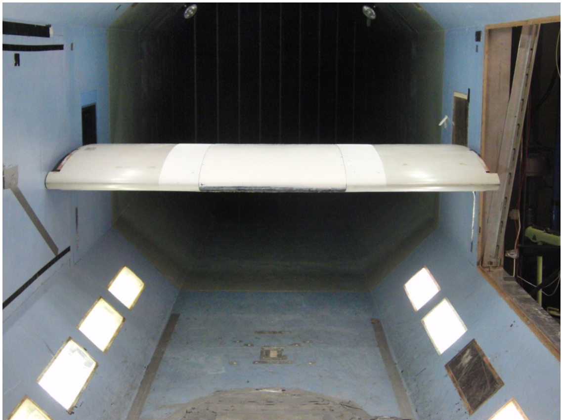
Figure 3-1 Fixed AOA model placed on the wind tunnel.
