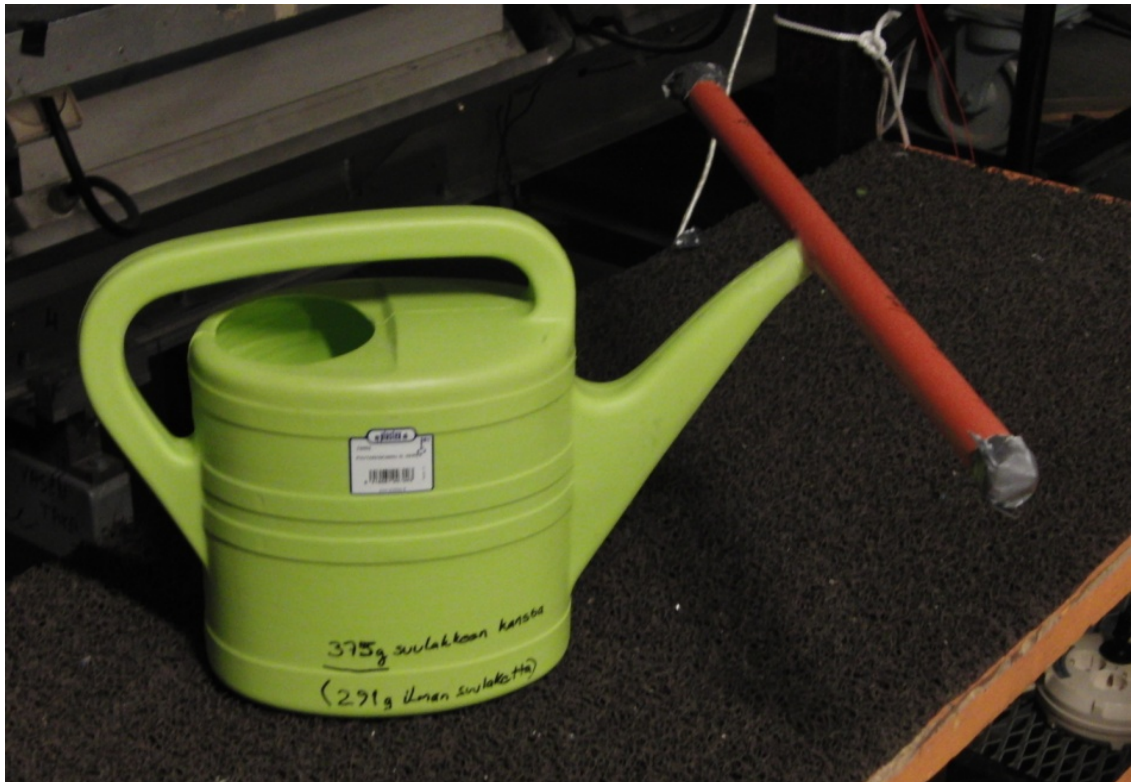
Figure 3-2 Watering can with a pipe-derived nozzle.
