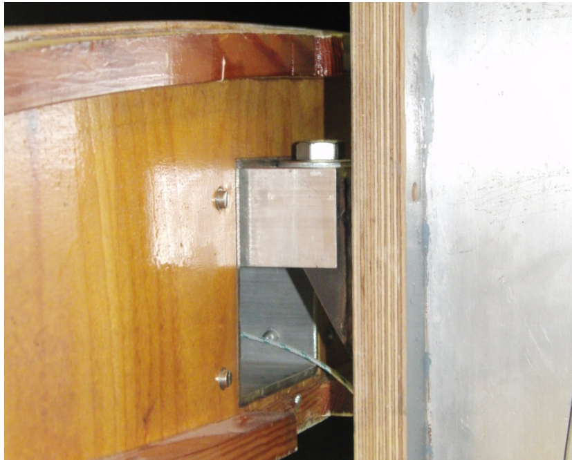
Figure A-2 Wing spar of the model placed on and fastened to the bracket. A thermocouple line led out of the model through the spar is also visible.
