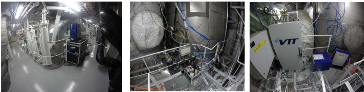
Figure 2.2. Left: Instruments at the engine out of ME2. Middle and right: Instruments before scrubber. For VTT's measurements, heated lines were used. For FMI and TUT measurements, a 10 mm Cu-tubing was used to transfer the diluted sample to upper level (after scrubber) for instruments that were not moved to lower level.
