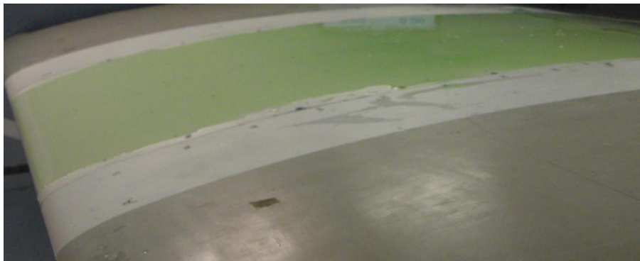
Figure 1. Wing section model in wind tunnel test section. Fluid applied to the test area of wing upper surface. Test area spans over 600 mm and extends from leading edge to trailing edge.
