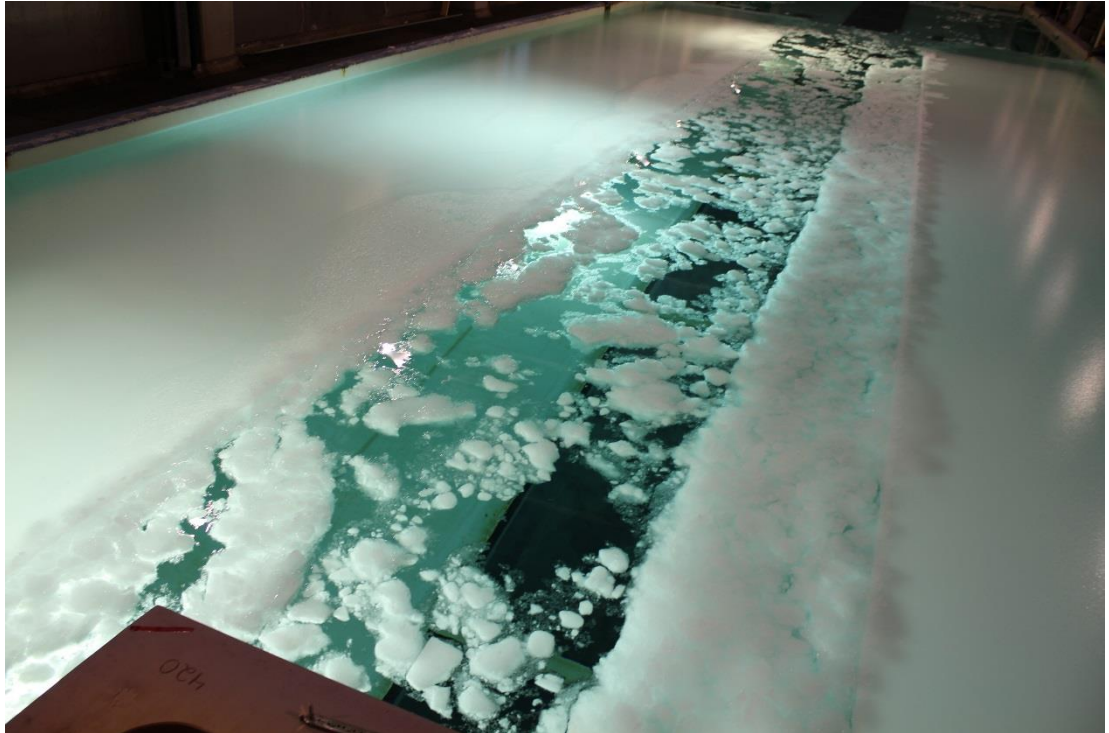
Figure 8-1 Channel behind the model, channel made of FGX ice, 500 kPa
