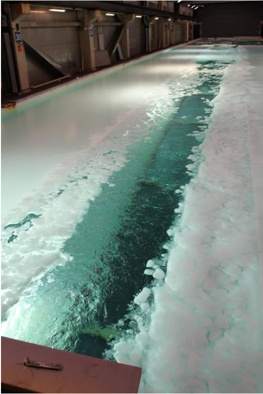
Figure 8-3 Channel behind the model in ice channel made of FGX-ice, 1000 kPa
