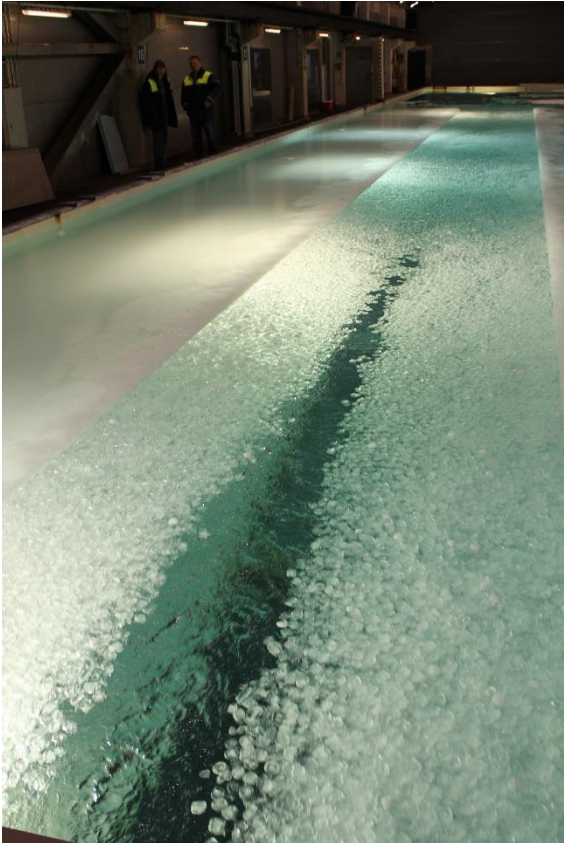
Figure 8-2 Channel closes nicely behind the model in ice channel made of ice cubes
