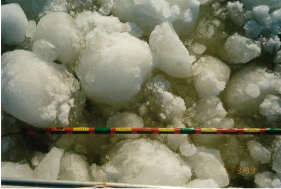
Figure 3-1: The Channel brash ice piece sample in the channel center line
