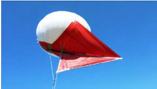
Figure 4 A 35 m 3 Allsopp Helikite in flight ( http://www.allsoophelikites.com/ )
