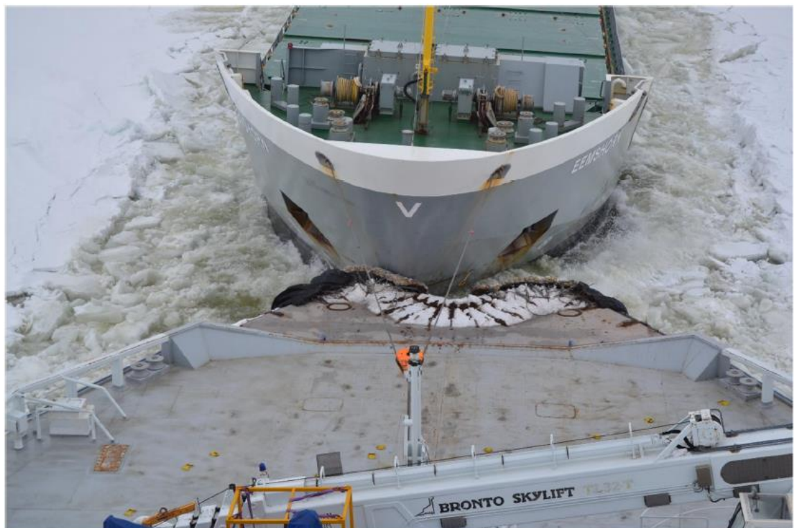
Figure 4-13. The arrangement of towing operations of “Eemshorn”
