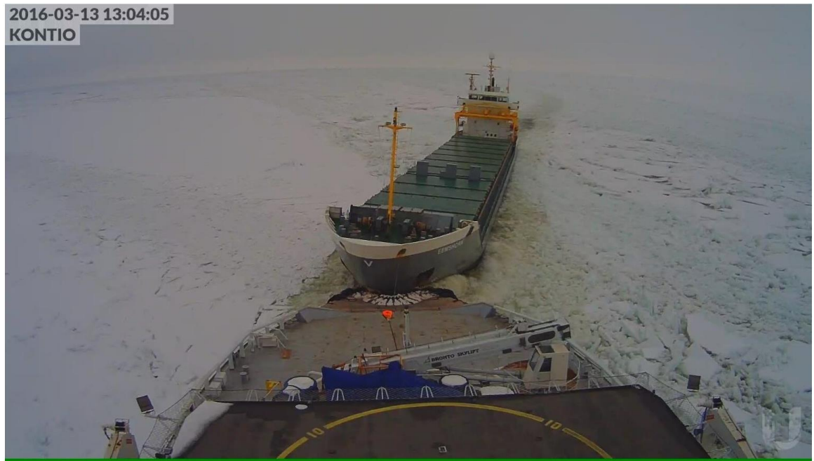
Figure 4-14. The towed vessel pushes the stern of the icebreaker
