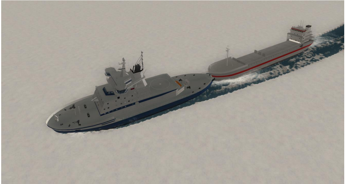
Figure 4-20. Towing in ice in the AAT ice simulator
