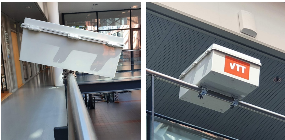
Figure 5: Radar enclosure with handrail fixtures.
