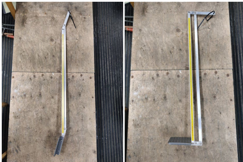
Figure 2. Ice thickness measurement stick with the perforated plate in straight and 90-degree angle orientation on the left and right, respectively.
