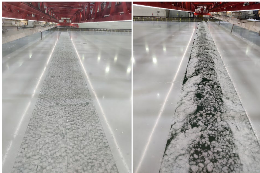
Figure 8. A typical brush ice channel produced from model ice on the left, and the channel after the tests.
