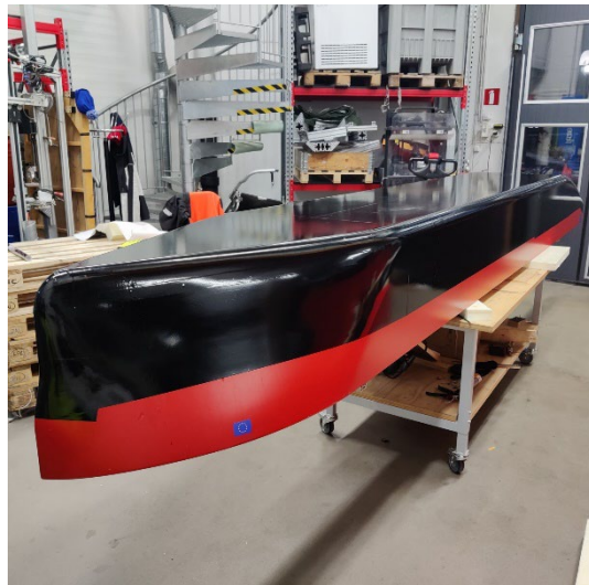
Figure 16. Infuture covered with D-C-fix contact plastic.
