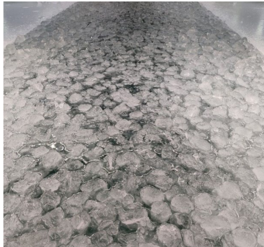
Figure 11. Ice cubes in the channel.
