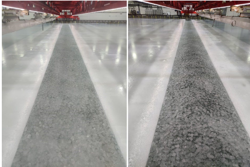
Figure 12. An ice cube channel before and after a test on the left and right, respectively.
