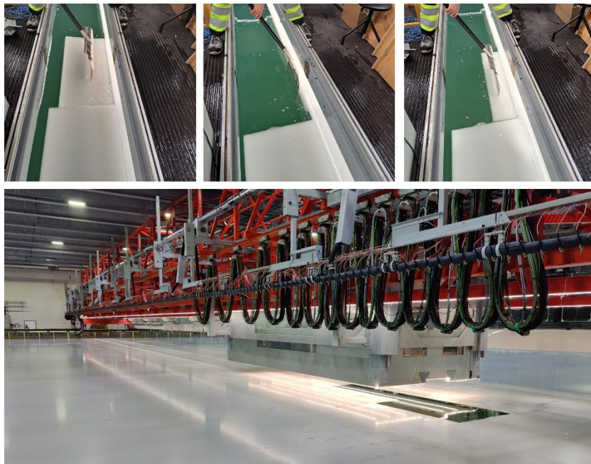
Figure 9. Channel preparation procedure for ice cubes.
