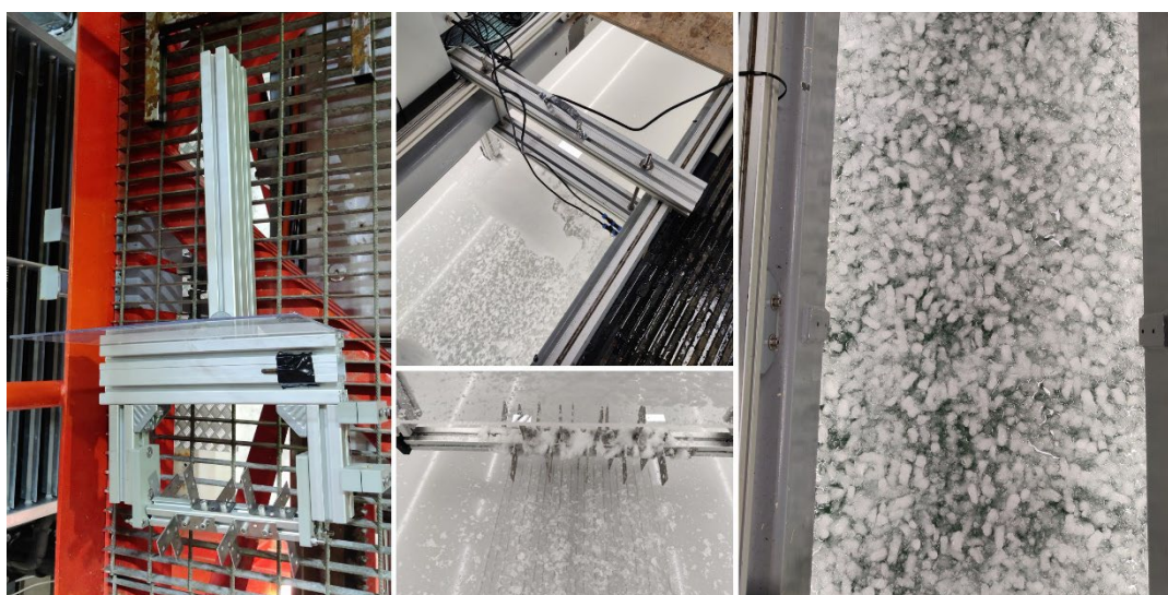
Figure 6. Brash ice hacking device on the left. The device attached to the carriage on the top centre, and the bar with brackets chopping ice on the bottom centre. Prepared channel on the right.
