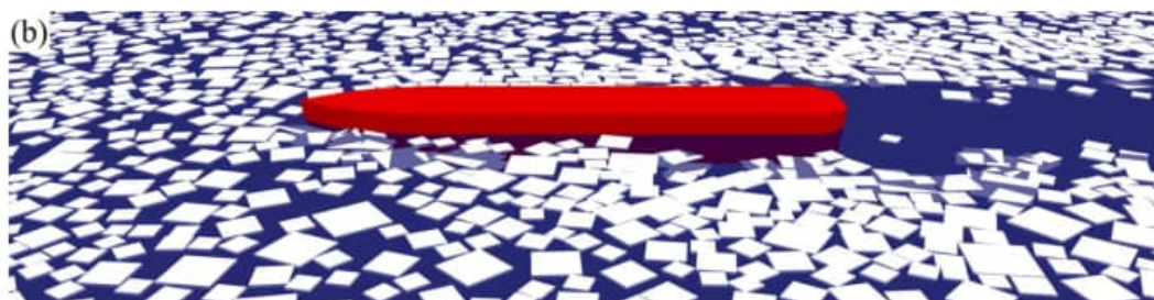
Figure 5: Ship in an ice floe field simulation by using the Aalto Ice Mechanics group's in-house DEM code, after Polojärvi et al. (2021).
